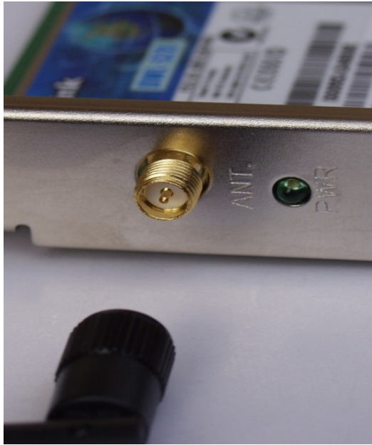
Image 20: A D-link PCI card with a RP-SMA female connector needs a pigtail or a converter in order to connect to a coaxial cable with a Heliax N-type male connector.
