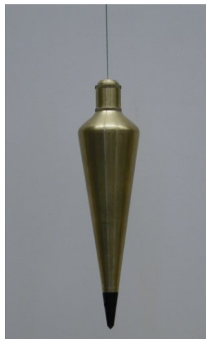
Image 16: A plumb bob used to adjust the guys in order to ensure a vertical tower.
