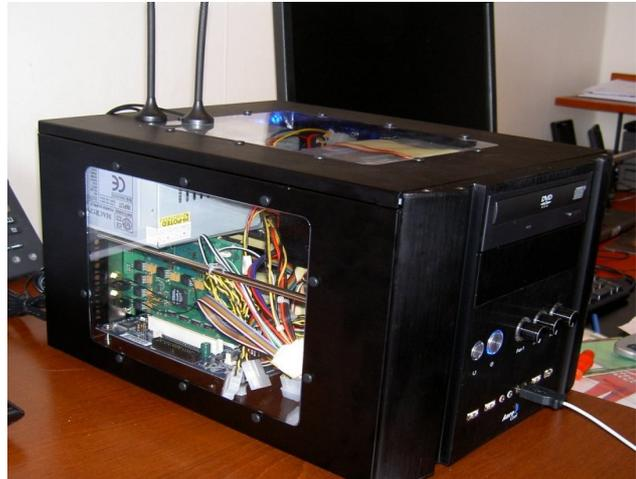
Apart from being able to handle SMSs, the sprinkler also acts as a complex audio mixer, capable of routing GSM calls to the traditional phone network or linking calls between different GSM operators. What makes the sprinkler attractive is its portability which enables the possibility of deploying a SMS server without the need of being directly connected to the operator's wired network.
